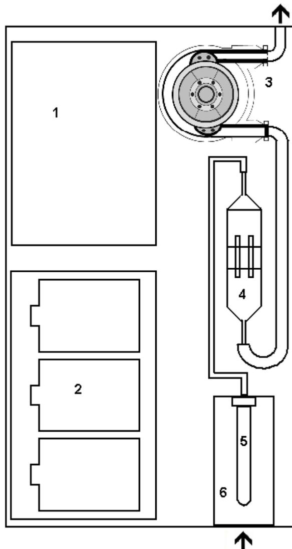
Continuous Flow Integrative Sampler (CFIS). An innovative device for time weighted average monitoring
