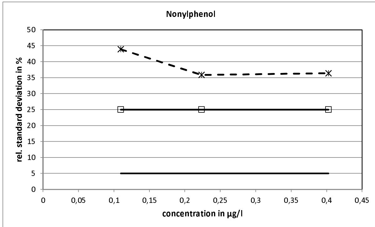
The relative standard deviation, derived from the Q-method, reached with all concentration levels the upper limit.
