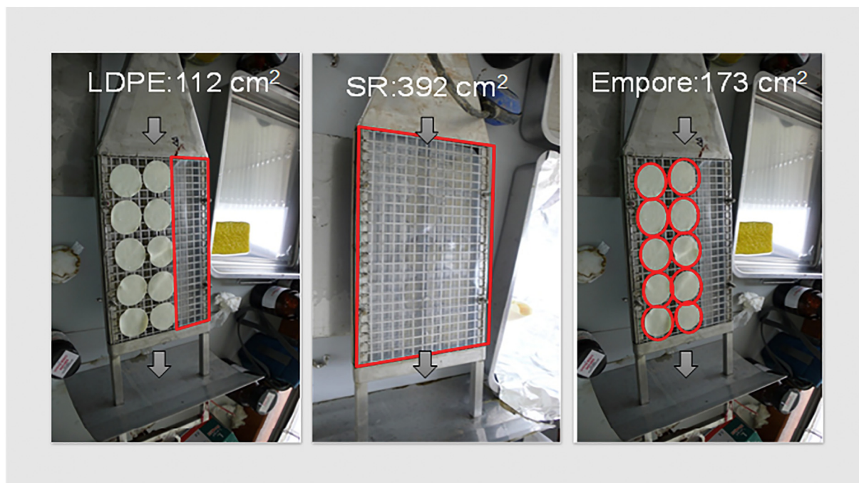
Fig. 1. Co-deployed AlteSil™ silicone rubber (SR sampler), SDB-RPS Empore disks (ED sampler) and LDPE stripes (LDPE sampler) in a DPS device. The arrows show the direction of water streaming through the exposure chamber.
